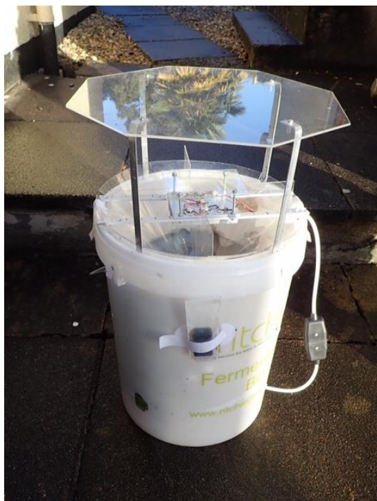
LED trap with rain guard fitted (left) and close up of LED array (below) (Mike Braid)
