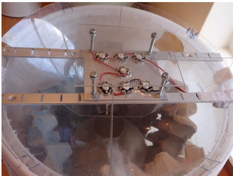
LED trap with rain guard fitted (left) and close up of LED array (below) (Mike Braid)
